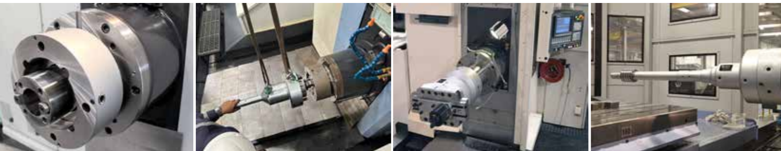
The bonnet securely bolts to the outer spindle of the machine.
